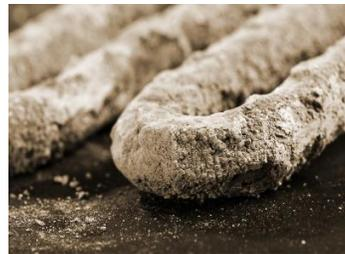
The three carbonates that form from the most common soluble metal ions are calcium carbonate, magnesium carbonate, and manganese carbonate. These three carbonates are very insoluble in water, tend to fall out of solution, and deposit as white to off-white crystals in pipes and on heating elements in hot water heaters, dishwashers, instant hot water heaters, and coffee makers.
